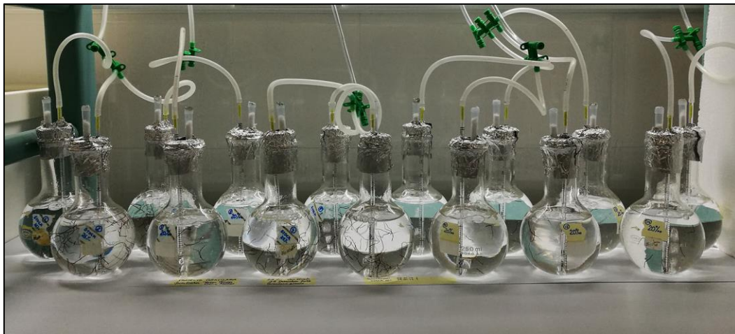
Figure 2.2: Culture setup of Gracilariopsis longissima assay at different salinities, assembled in a climatic room (24 ± 1°C) with photoperiod set at 12:12 (Light:Dark) and provided by daylight cool white fluorescent lamps (10-15 μmol photons m -2 s -1 ).
