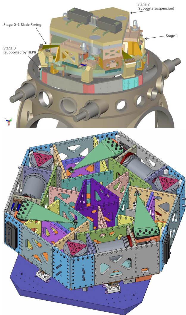
Figure 3.14: CAD rendering of the BSC-ISI (top) installed in its vacuum chamber. Top view of the HAM-ISI isolation stage (bottom) with the table top removed to show the placement of major components .
