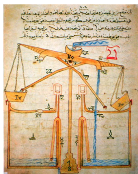
Figure 1.1 : Water Raising Device of Al-Jazari.
