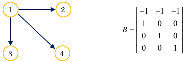
Figure 5.2: A formation of 4 robots and related incidence matrix
