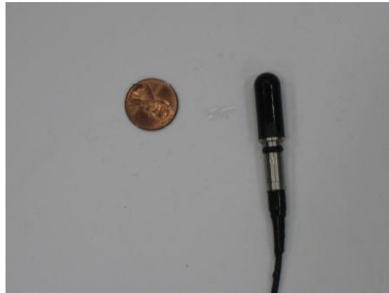
Figure 49 - The Scout: an Hydrophone
