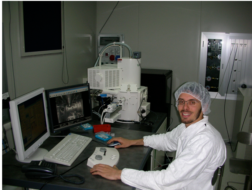
Figure 3.3: Picture of the EBL instrument in the NEST laboratory, also used for scanning electron microscopy.
