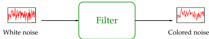
Figure 34: Generation of a colored noise sequence
