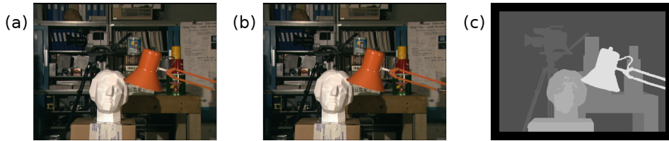
Figure 2.5: A pair of rectified images (a), (b) and the corresponding disparity map (c).
