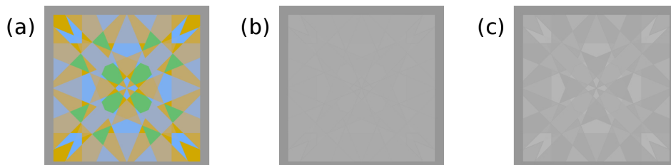
Figure 3.1: An isoluminant color image (a) converted with the CIE Y method (b) and with the Fairchild Lightness method (c).
