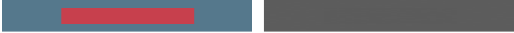
Figure 1.1: Isoluminant changes are not preserved with traditional color to grayscale conversion. Converting an image of a reddish rectangle whose luminance matches that of the blue background to grayscale results in a featureless image.
