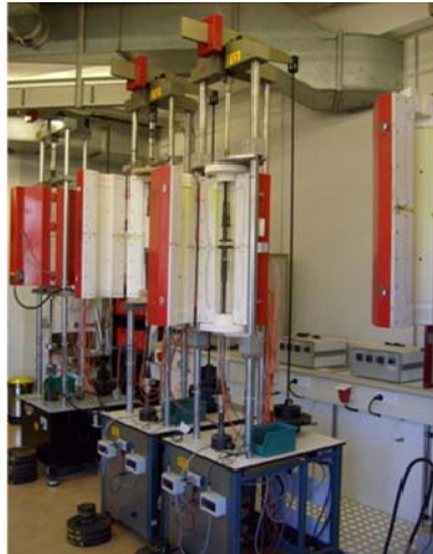
Fig. 4.12 Uniaxial Creep testing devices (JRC-IE lab)
