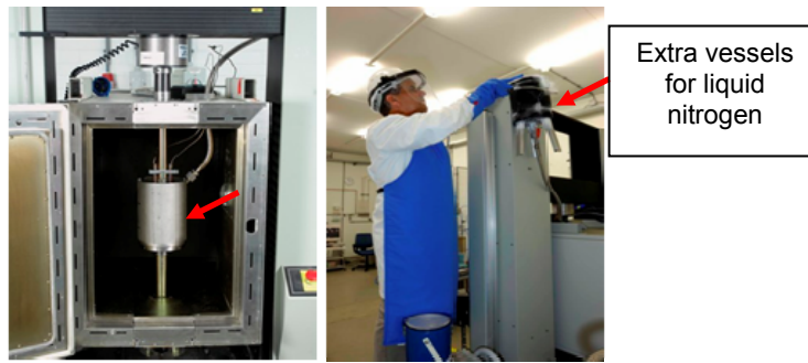
Fig. 4.8 Liquid Nitrogen cooling system used for temperature of -192^{\circ}\text{C}
