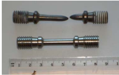
Fig. 4.22 Uniaxial creep sample – before and after the testing
