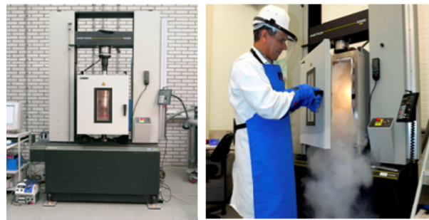
Fig. 4.7 SP fracture equipment with environmental chamber mounted
