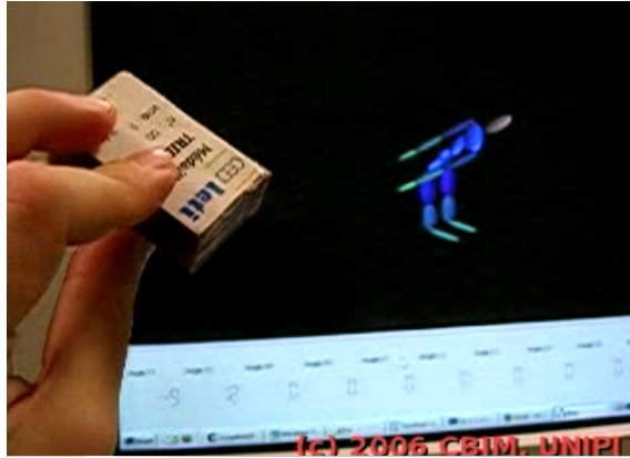
Figure 2.6: Use of Inertial Measuring Units (IMU) in posture reconstruction (CBIM-UNIPI, Italy).
