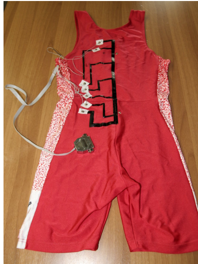
Figure 3.1: The sensorized prototype realized on a rowing Lycra suite.
