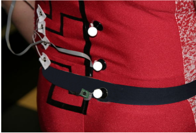
Figure 3.9: Sensorized prototype with CEs, accelerometers and Elite (BTS, Italy) optical markers.
