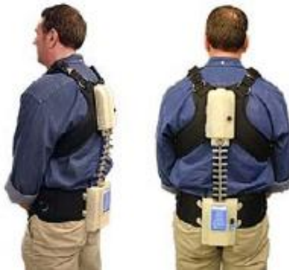
Figure 2.5: The Lumbar Motion Monitor system (LMM, Chattecx Corp. USA).
