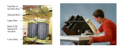
Figure 7.5: Prototype of robotic arm composed by 4 bundles of actuators, each of them composed by 64 fibers.
