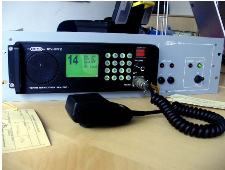
Figure 2.6: Elman RTV-1077-D VHF-DSC transceiver (front panel)
