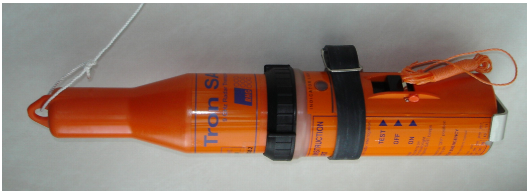
Figure 2.3: An installed radar SART
