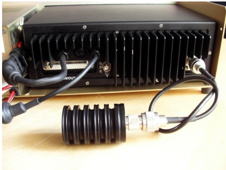
Figure 2.7: Elman RTV-1077-D VHF-DSC transceiver (rear panel)
