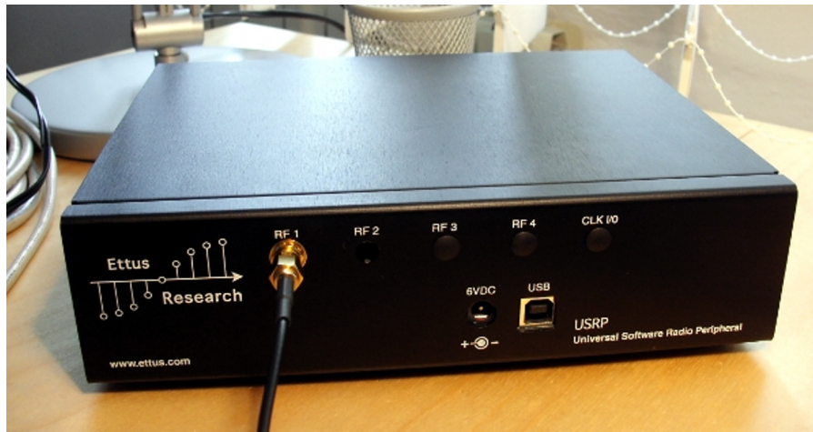
Figure 1.9: USRP enclosure: daughterboards connectors replicated on front panel.
