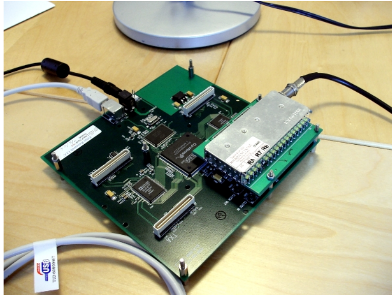
Figure 3.2: The VHF receiving interface (an USRP with TVRX daughterboard)
