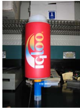
Figure 5.12 Modified container to chill the R-Tube
