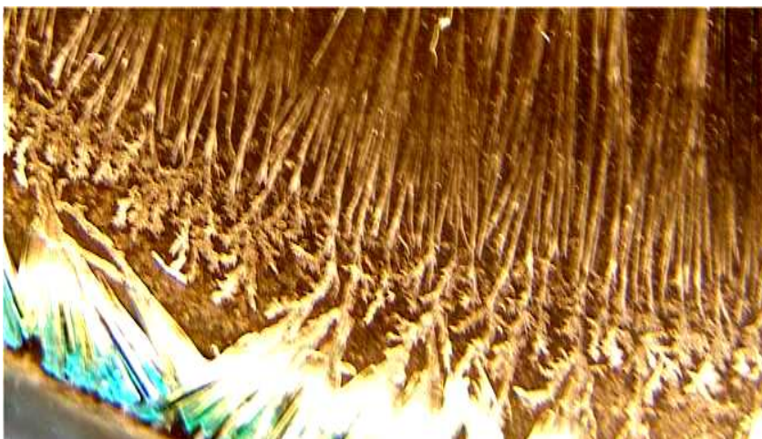
Picture 19: Example of a poor peripheral zone. The dendritic shapes are less ramified. There are more free spaces inside the peripheral zone. The connection to the copper chloride zone becomes weak.
