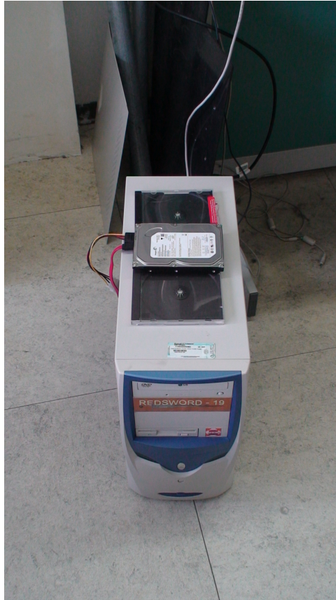
Figure 3.3: The test setup for Soft-DVB's first draft. The 7200rpm Seagate Barracuda disc is visible on top of the pc
