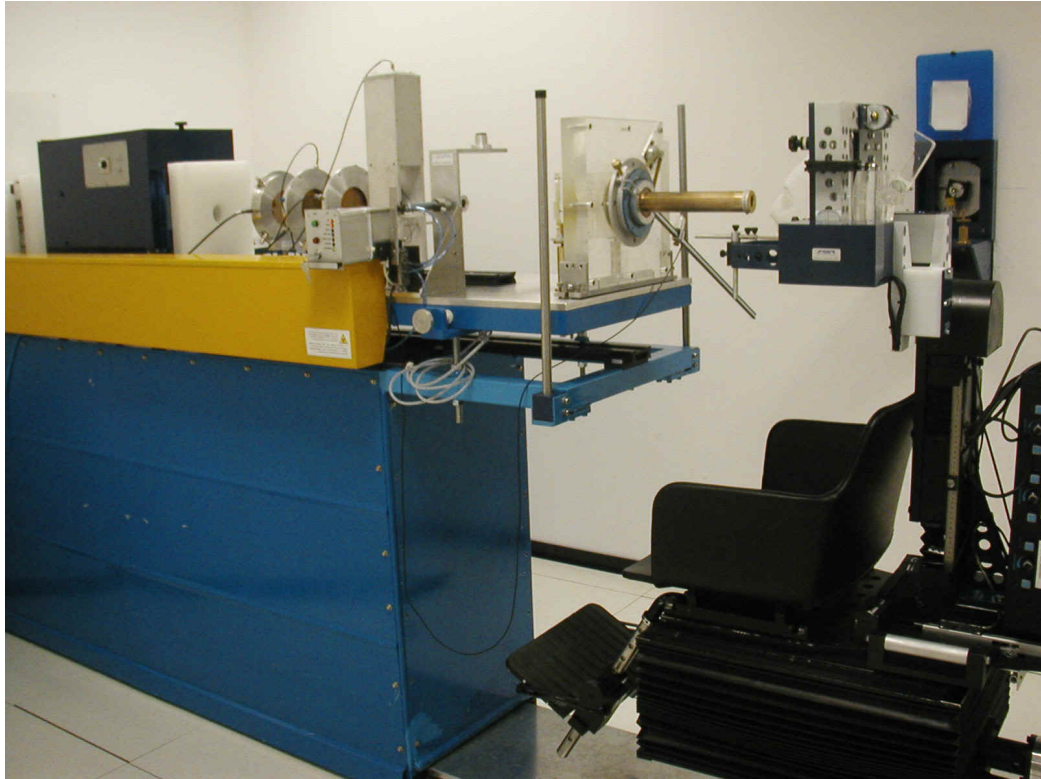
Figure 2.9: View of the treatment room at CATANA. For measurements on plastic phantoms the chair shown in the figure is replaced by the aluminum table shown as element 3 in figure 2.8.
