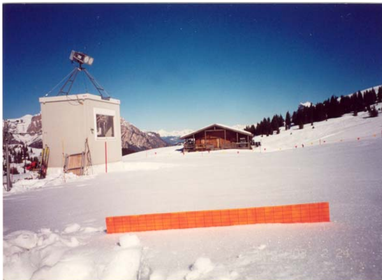
Fig. 38 – The microwave instruments shelter placed on the Mount Chertz test site during the 2002/2003 winter season. In the foreground it is possible to see a profilometer for the roughness measurements
