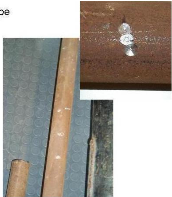
Figure 5-3 Defect growth (negative stepwise) in a 2" steel pipe
