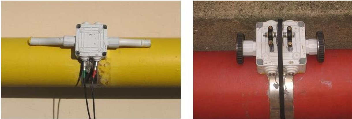
Figure 7-4 Local Acquisition Sensor for UGW: 1 st and 2 nd version
