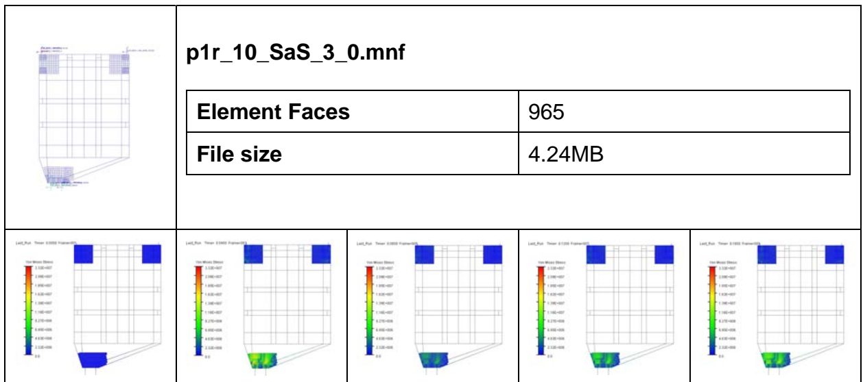
Figure C.3-2: Stresses in a Spot-mesh model
