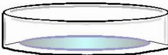
Figure 3.5. Test sample assemblage in glass Petri dishes for thermal aging in air ventilated oven
