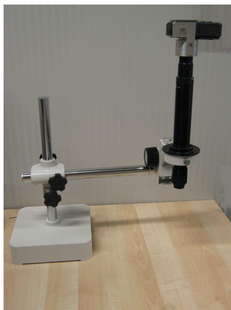
Fig. 31 – Photo of the home-made system used for acquiring digital optical images.
