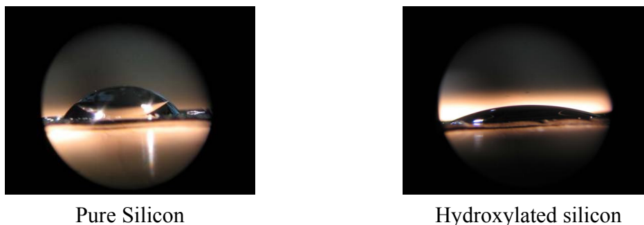
Fig. 88 – Optical microscope images of distilled water droplets on pure silicon (left) and on hydroxylated silicon (right).
