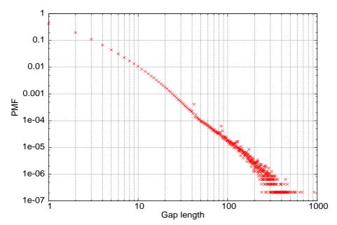
$\textbf{Fig. 8.6.} \ \ \textbf{Probability mass function of gap length at frame level}.$
