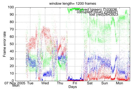
${\bf Fig.~8.3.~} \ {\bf Average~of~received,~lost~and~corrupted~frames~during~the~second~week.}$
