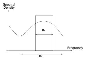
Fig. 3.6. Flat-fading case:  $B_s$  is the signal bandwidth, and  $B_c$  is the coherence bandwidth
