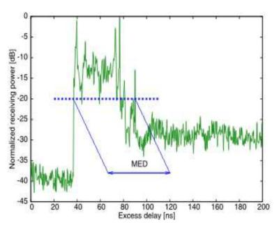
Fig. 3.13. Maximum excess delay
