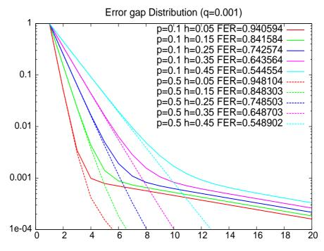
Fig. 5.2. Error gap distribution for the Gilbert model.
