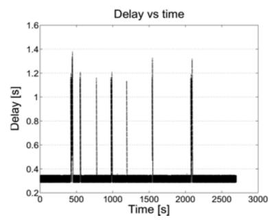
Fig. 2.2. Typical trend of packet delay for the satellite channel in 45 minutes of transmission.
