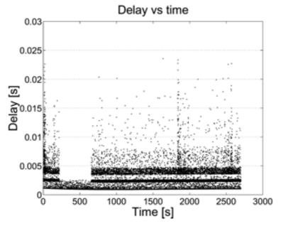
$\bf Fig.~2.9.$  Typical trend of packet delay for the WLAN channel with Retry 7 in 45 minutes of transmission.
