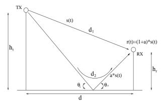
Fig. 4.1. 2-ray ground reflection model.
