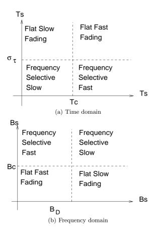
Fig. 3.11. Type of small-scale fading types of experienced by a signal from the viewpoint of (a) symbol period, (b) baseband signal bandwidth.
