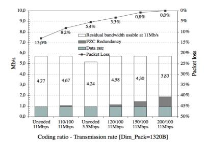
Fig. 2.20. Redundancy and error correction performance vs. coding ratio for client A.
