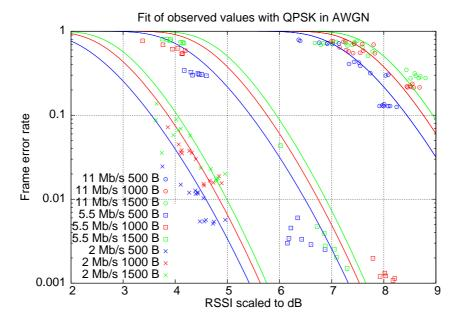
Fig. 7.8. Fit of Equation 7.10 with measured values.
