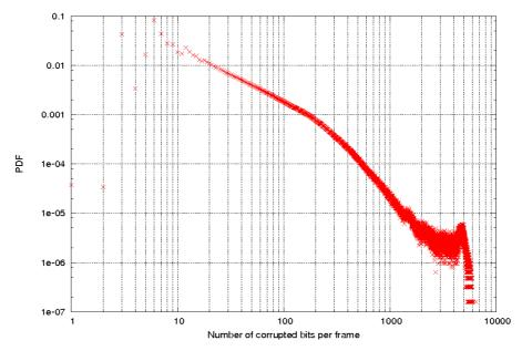
${\bf Fig.~8.9.}$  Probability mass function of number of errored bits per frame
