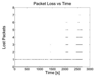
Fig. 2.17. Lost packets for the full path video stream.
