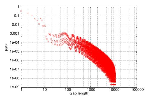
$\textbf{Fig. 8.7.} \ \ \textbf{Probability mass function of gap length at bit level}.$
