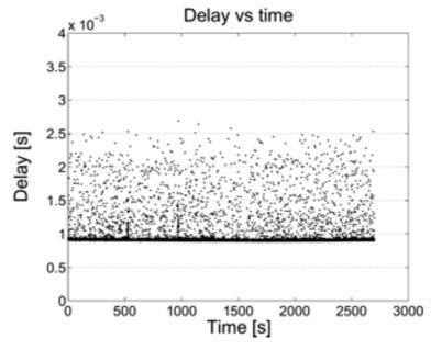
**Fig. 2.6.** Typical trend of packet delay for the WLAN channel with Retry 0 in 45 minutes of transmission.
