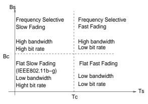
Fig. 3.12. Types of small-scale fading for the IEEE802.11 signal
