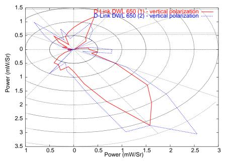
Fig. 7.3. Horizontal radiation pattern for two PCMCIA cards (vertical polarisation).
