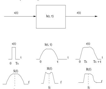
Fig. 3.9. Frequency selective fading channel characteristics
