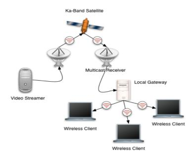
Fig. 2.18. The test-bed network topology.
