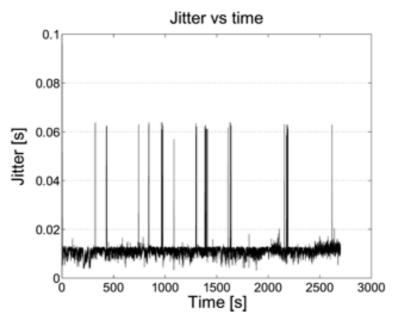
Fig. 2.16. Packet jitter for the full path video stream.
