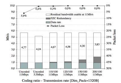
Fig. 2.21. Redundancy and error correction performance vs. coding ratio for the client B.
