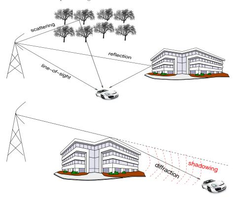
Fig. 3.1. A typical scenario of mobile radio communications
