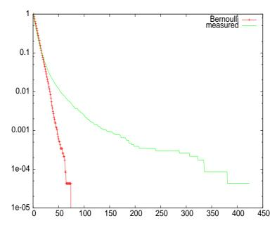
Fig. 9.2. Error gap length distributions for one observed frame error trace and a synthetically generated Bernoulli trace with the same average frame error rate.
