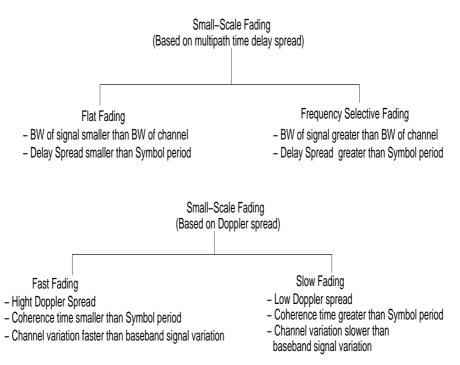
Fig. 3.10. Type of small fading
