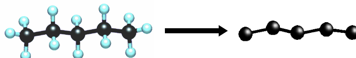
Figure 2.1: The chain is described as a sequence of beads, where each bead represents a single methylene \text{CH}_2 group. No distinction is made between internal methylene \text{CH}_2 groups and terminal methyl \text{CH}_3 groups [120].
