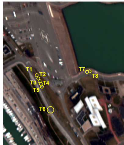
Figure 4.2. Ground truth of the collected HSI. The anomalous changes ( deletions ) are highlighted with yellow circles: two vehicles in the top right, five vehicles in the top left and one vehicle in the middle left.
