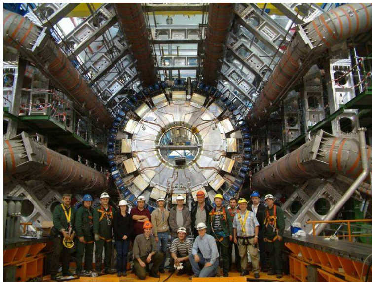
Figure 2.9: TileCal barrel at the interaction point. The cryostat with the front-end electronics for EM calorimeter is visible in the inner part. TileCal is surrounded by the 8 superconducting magnets for the muon toroid system.
