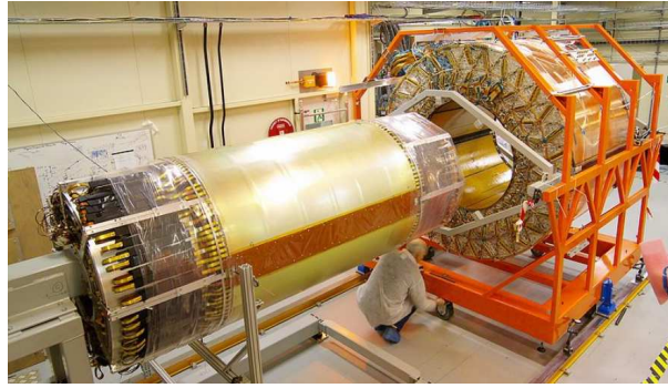
Figure 2.8: ID Barrel integration: SCT (left) being inserted in the TRT.
