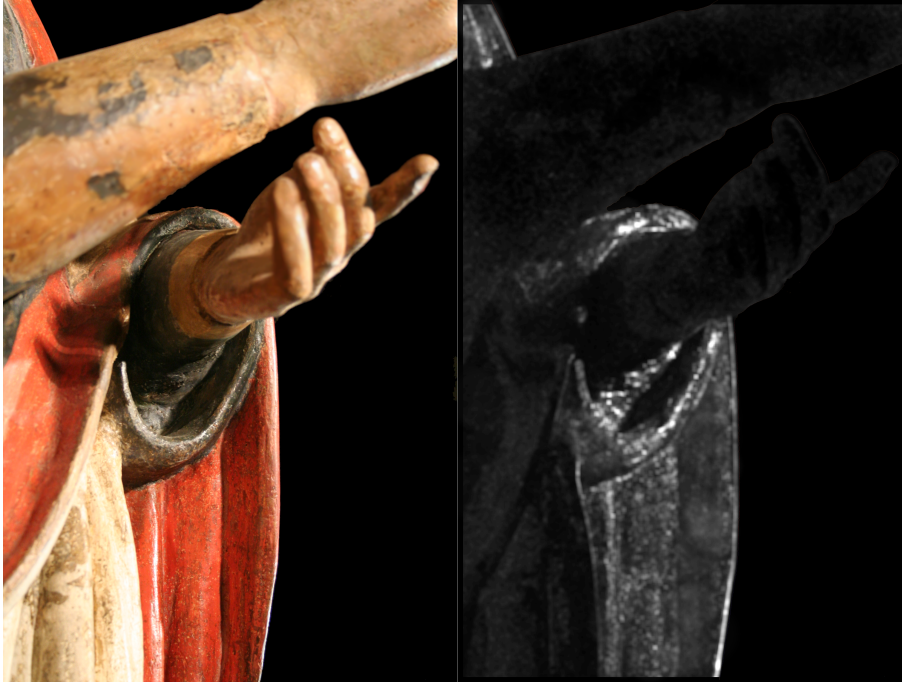
Figure 3.3: Focus masking example. An image of the wooden statue with large depth extent. As detected by the focus mask, the hands are out of focus due to depth of field, while the red part of the vestment is perfectly focused.
