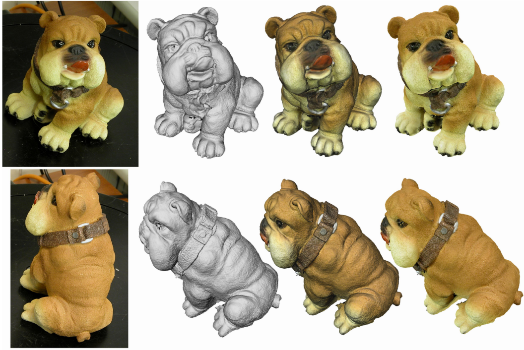
Figure 3.4: An example of per-vertex color mapping. The 3D model is composed by 1 million triangles, with a mapped photographic dataset of 8 images 2560 \times 1920 . From left to right: original photos, geometry, color+shading, color only.
