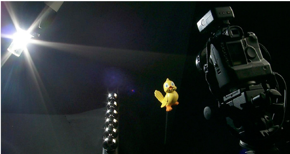
Figure 2.10: BRDF acquisition using Lensch et al. method [85]: the sampled object is illuminated with a strong quasi-punctual light source, the surface response is captured using a digital camera. Both light and camera position are calculated using the mirroring spheres
