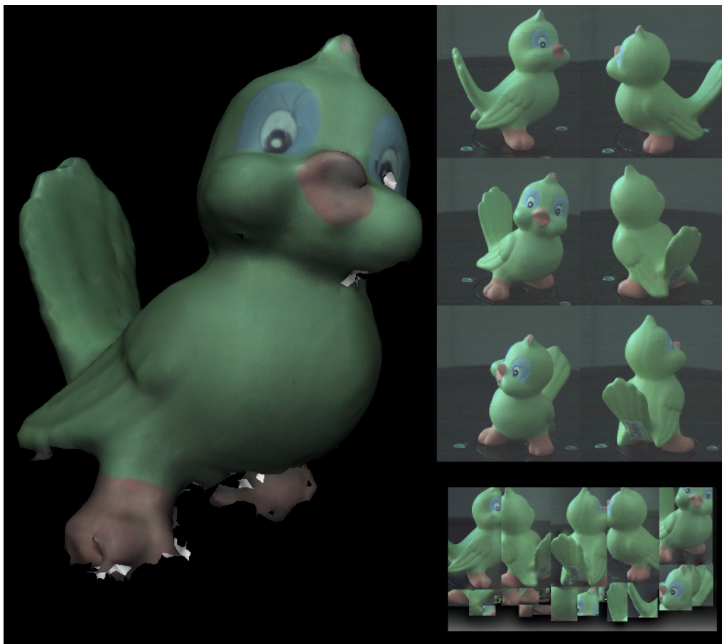
Figure 2.5: Texture Mapping Example. Results obtained using our algorithm [21]. On left the textured 3D model, on upper right the input images, on lower right the texture image
