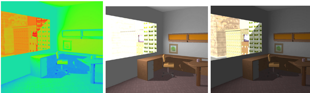
Figure 2.6: High dynamic range imaging. Left: HDR luminance represented in false colors raw geometry. Middle and Left: from the HDR data, images with different exposures can be generated
