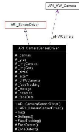
Figure 3.12: Architecture of the CameraSensorDriver structure. The hardware abstraction is gained through the HW_Camera structure
