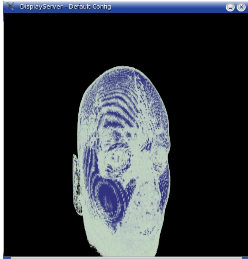
Figure 5.5: MRI scan of a human head. The data set is of 256^3 voxels. Each voxel is originally stored with 8 bits. The rendering is accomplished using 4 rendering nodes. Data set source: http://www9.cs.fau.de/Persons/Roettger/library/
