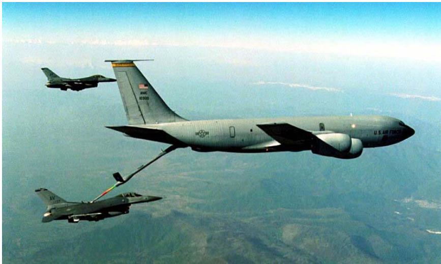
Fig. 1.1: aerial refueling using a boom system
