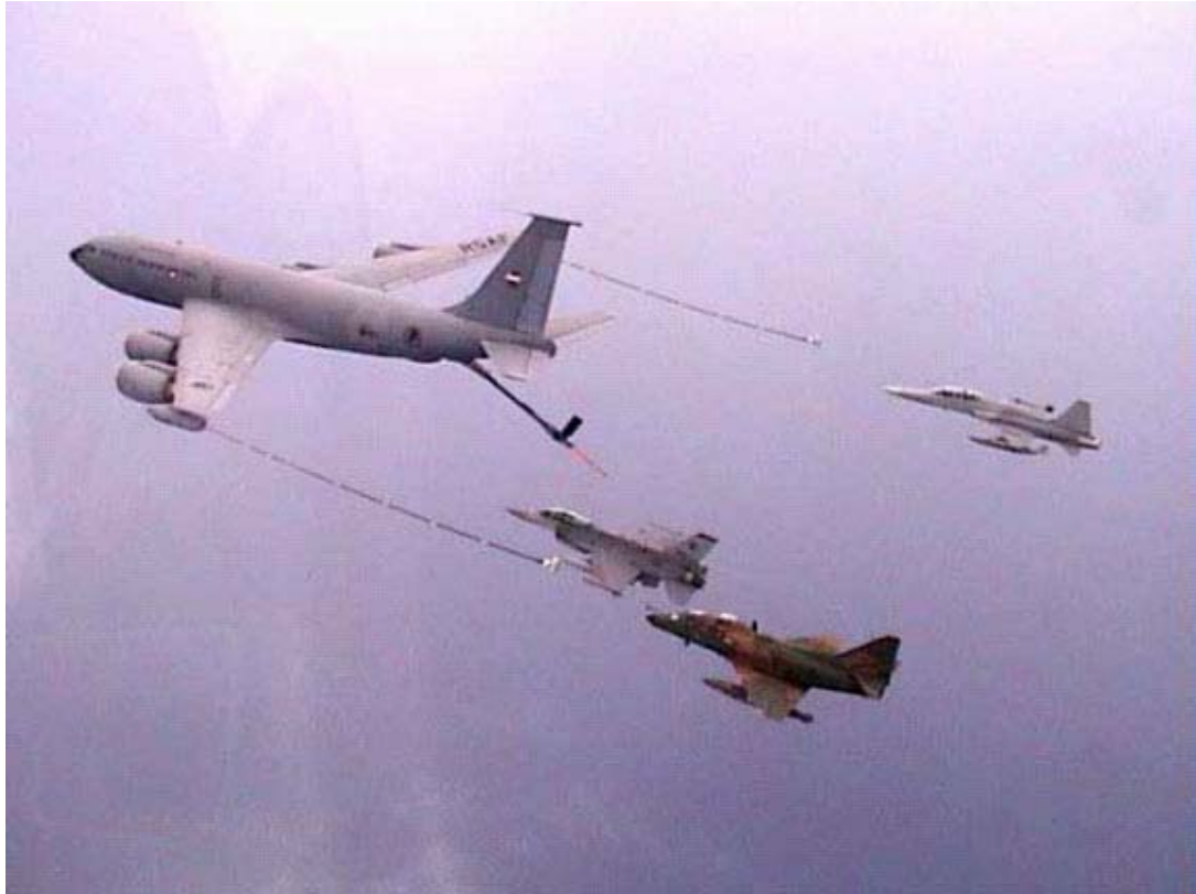
Fig. 1.2: aerial refueling using a probe and drogue system
