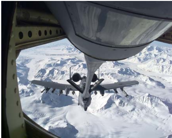
Fig. 2.6: Boom operator view in a real and simulated refueling maneuver
