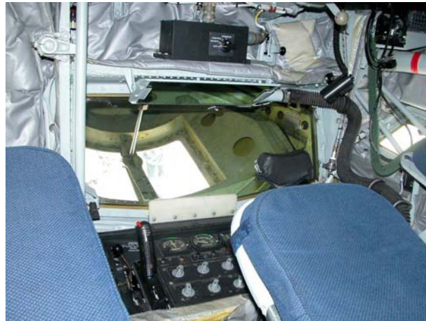
Fig. 2.5: Boom operator console
