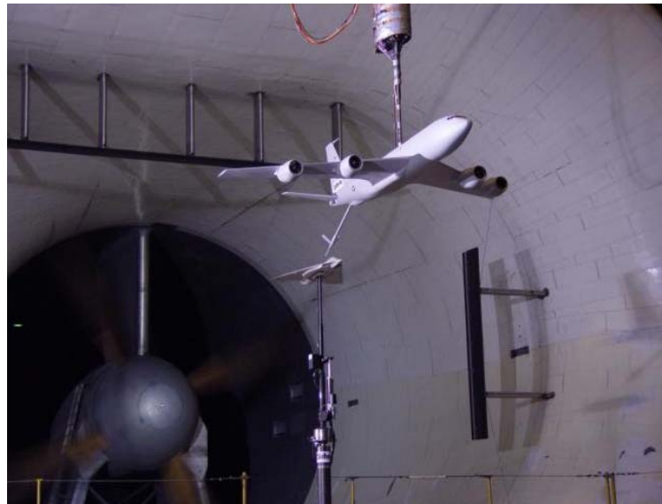
Fig. 3.9: AAR test to search the coefficient increment
