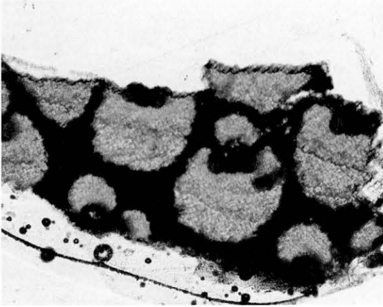
図102 刳足裏側補強材のクロスセクション—竹または笹 Cross section of the reinforcing material on the inner side of the kuroshitsu - bamboo or wild bamboo
