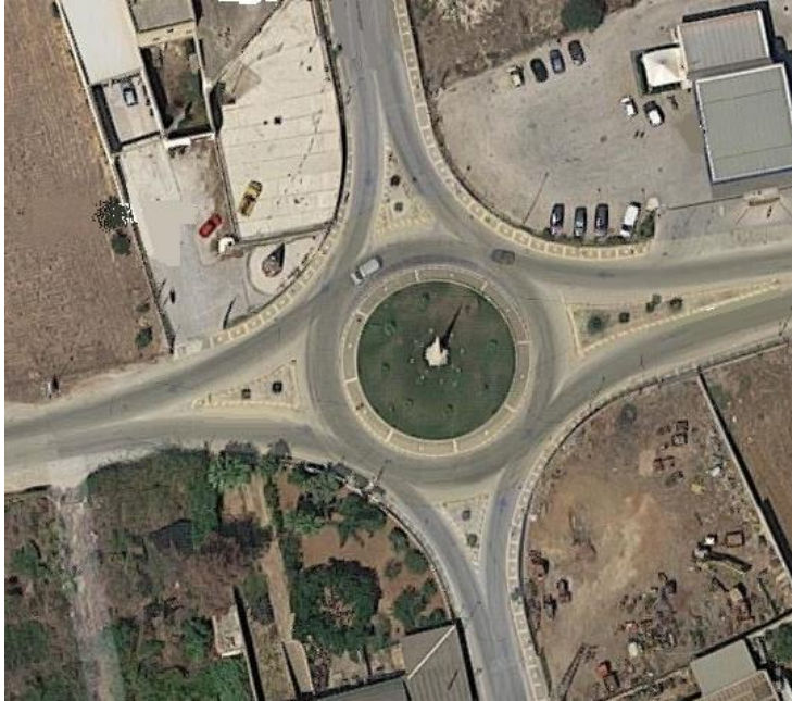
Figure 3 An example of single-lane roundabout located in Mazara Del Vallo, Trapani, Italy, from Google
