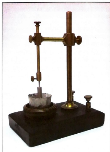
Fig. 4 The silver voltmeter, after the restoration and assembling work.
