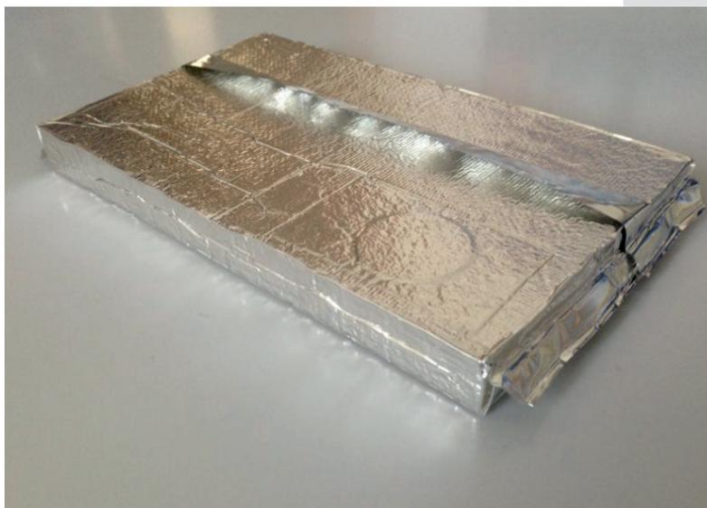
Figure 1. VIP Panel with silica core and aluminium outer laminate.
