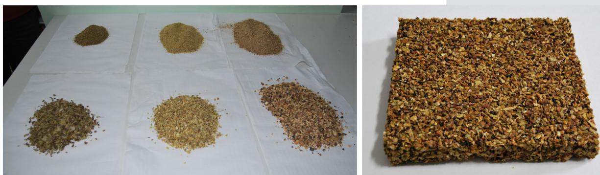
Figure 5. Granules sorted by size and assembled in panel.
