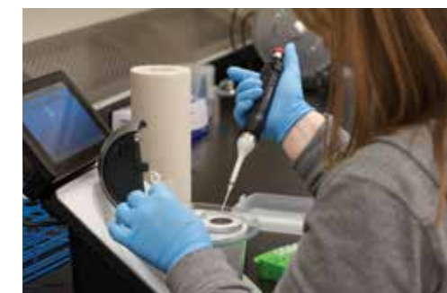
Behavior Core Manager Ivy Bergquist, B.S., RLATg, uses the Nanodrop spectrophotometer to quantify ribonucleic acid (RNA) concentrations in a sample.
