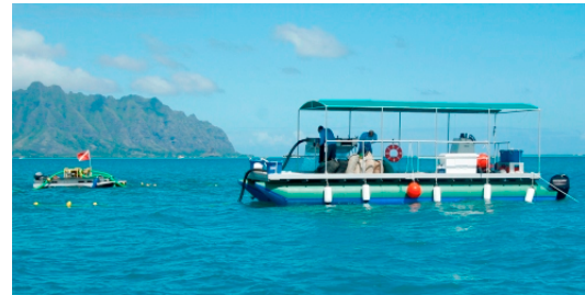
Figure 6. The barge made by the Nature Conservancy to vacuum the invasive algae species from the water. (The Nature Conservancy 2014).
