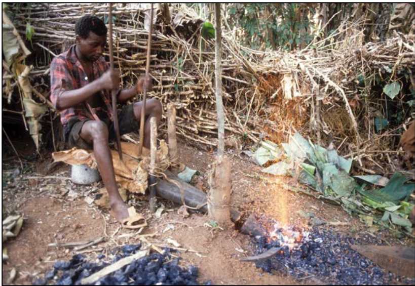
A young blacksmith in the Ituri works the bellows, making the fire hot enough to soften a recycled metal truck spring such that it can be hammered into an axe blade. While the blade is still red hot, it will be inserted into an axe handle crafted from a specific forest species, the sap of which acts as a sort of glue.
