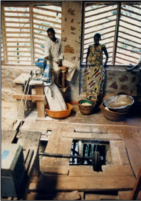
Microhydro mill near Loko. Through a series of belts and pulleys, the turbine (below flooring) runs a variety of machines including maize and manioc grinders and coffee hullers. A woman waits for her maize to be ground into flour, a process traditionally done with mortar and pestle.
