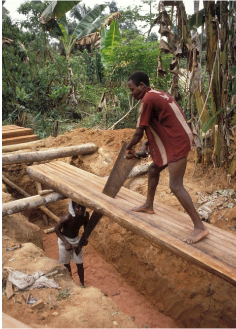
Two men produce pit-sawn mahogany lumber in the Ituri. The tree, located directly behind a village homestead, had died while standing and was subsequently felled. Such hand-sawn operations have long served as a sustainable method of harvesting timber for local needs.
