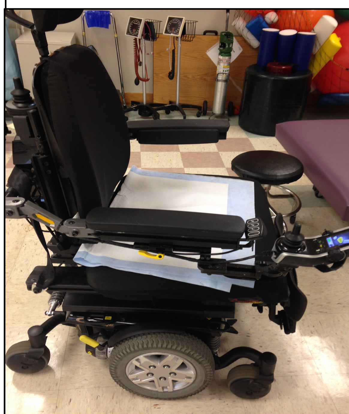
Figure 2a. Power wheelchair used for long distance mobility
