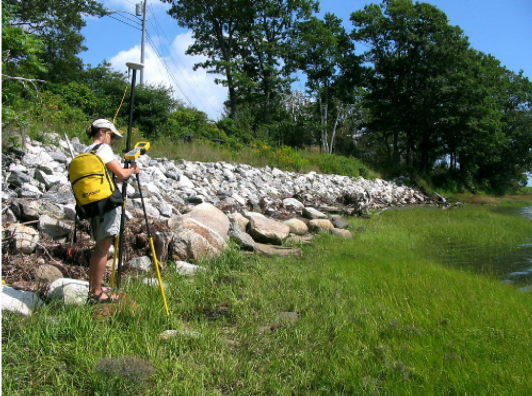
Figure 2. Mapping fringing salt marsh site with GPS.
