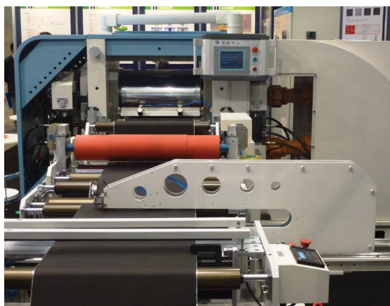
Fig. 4. Calander (pressing) machine for lithium-ion battery electrode manufacturing (by RudolfSimon, via Wikimedia Commons).
