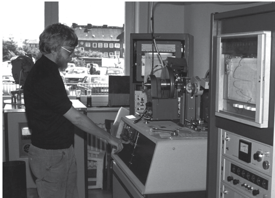
Fig. 2. X-ray diffractometer Philips PW1050 at the Geological-Paleontological Institute, Kiel; user: Prof. Dr. Dietmar Schenk (by Hannes Grobe/AWI, via Wikimedia Commons).
