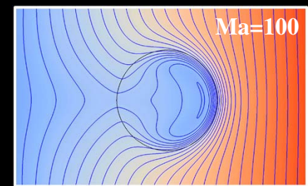
Temperature distribution in proximity to the droplet
