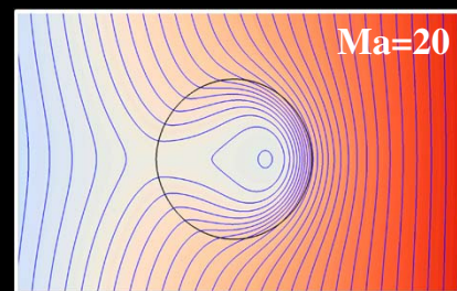
Temperature distribution in proximity to the droplet
