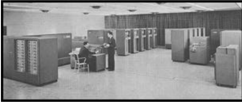
Figure 1.1: IBM computer in 1955, capable of performing 3750 operations per second. Total memory of approximately 10 kbytes.
