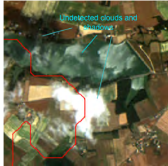
Figure 2.3.: Example of incomplete mask of clouds. The red lines correspond to the contours of the cloud mask [Hagolle et al., 2010]
