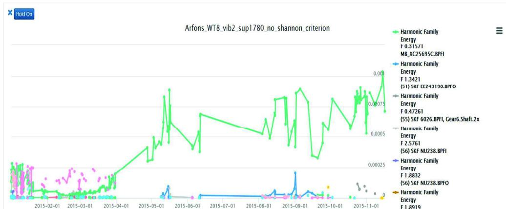
**Figure 9: trend of the energy feature of every harmonic family associated to a bearing. The faulty bearing is in ocher.**
