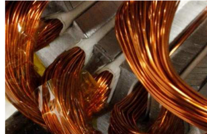
Figure 19. Detail of phase-to-ground insulation.
