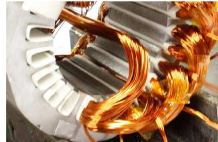
Figure 12. Details of turn distribution during coils insertion
