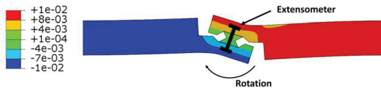
Fig. 2 : Residual rotation and axis of measurement of spreading u (mm)
