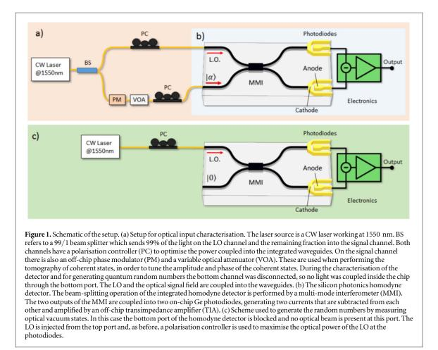
single photon level—by measuring the field's interference with a bright laser, that acts as a local oscillator (LO), at an optical beamsplitter. Ideally, measurement of the difference in the photocurrents in the two photodiodes is proportional to the quantum quadrature operator
