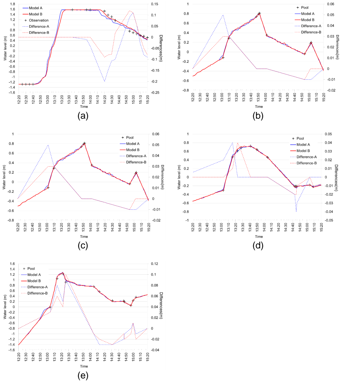
509 Figure 10 Observed and modelled water level hydrographs of the 23 July 2015 event 510 at WL gauge (a), at the outlet detention pools of Networks 1 to 4 (b-e, respectively).
