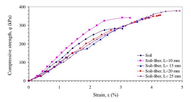
Fig. 2. Stress-strain curves for natural soil and reinforced soil with 0.5% fiber and different lengths
