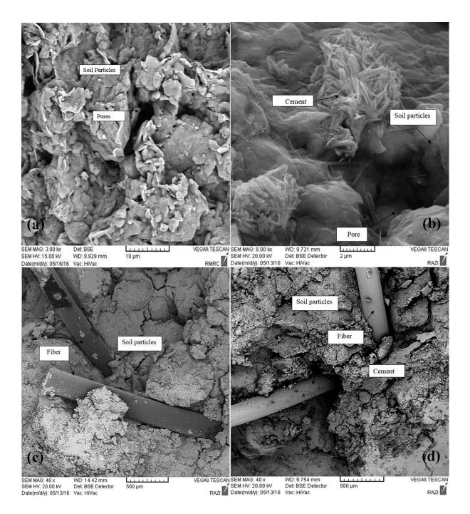
**Fig. 13** Scanning electron micrograph of (a) natural soil; (b) soil+8% cement, (c) Soil+1% fiber with length 10 mm; (d) Soil+8% cement +1% fiber with length 10 mm
