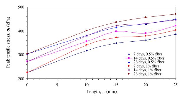
Fig. 12. Variations of peak tensile stress against length of fiber for reinforced soilcement samples with 10% and 0.5 and 1.0 % fiber inclusion at different curing times
