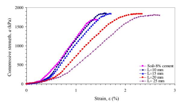
**Fig. 4.** Stress-strain curves for soil-cement and reinforced soil-cement with 8% cement and 0.5% fiber for curing time of 7 days
