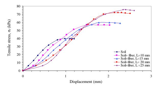
Fig. 8. Tensile stress-displacement for soil and soil reinforced with 0.5 % fiber at different lengths
