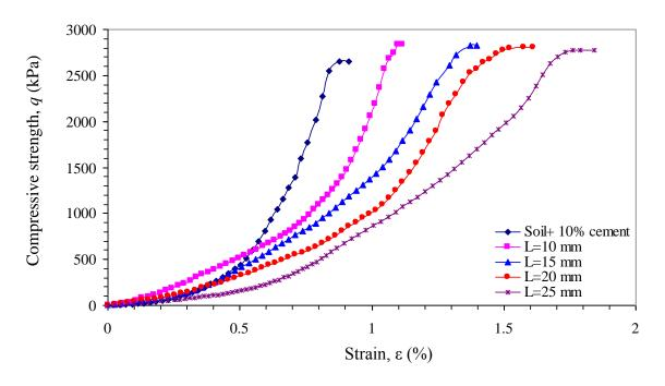
**Fig. 5.** Stress-strain curves for soil-cement and reinforced soil-cement with 10 % cement and 0.5% fiber for curing time of 28 days
