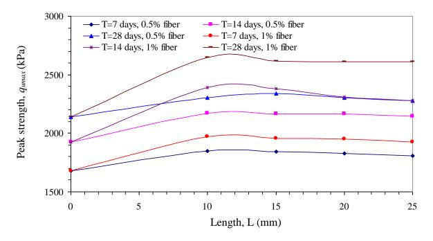
**Fig. 6.** Variations of peak strength against length of fiber for soil-cement with 8 % cement and fiber inclusion 0.5% and 1% at different curing times
