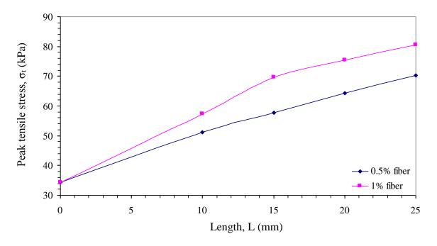
Fig. 10. Variations of peak tensile stress against length of fiber for reinforced soil samples with 0.5 and 1% fiber content
