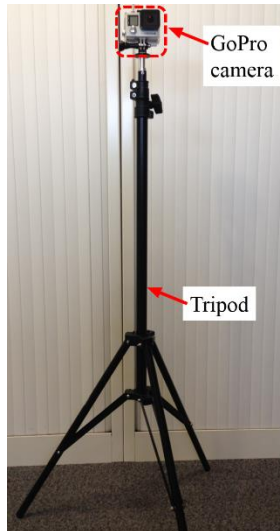
Figure 1 Hardware of vision-based system consisting a GoPro Camera and a tripod
