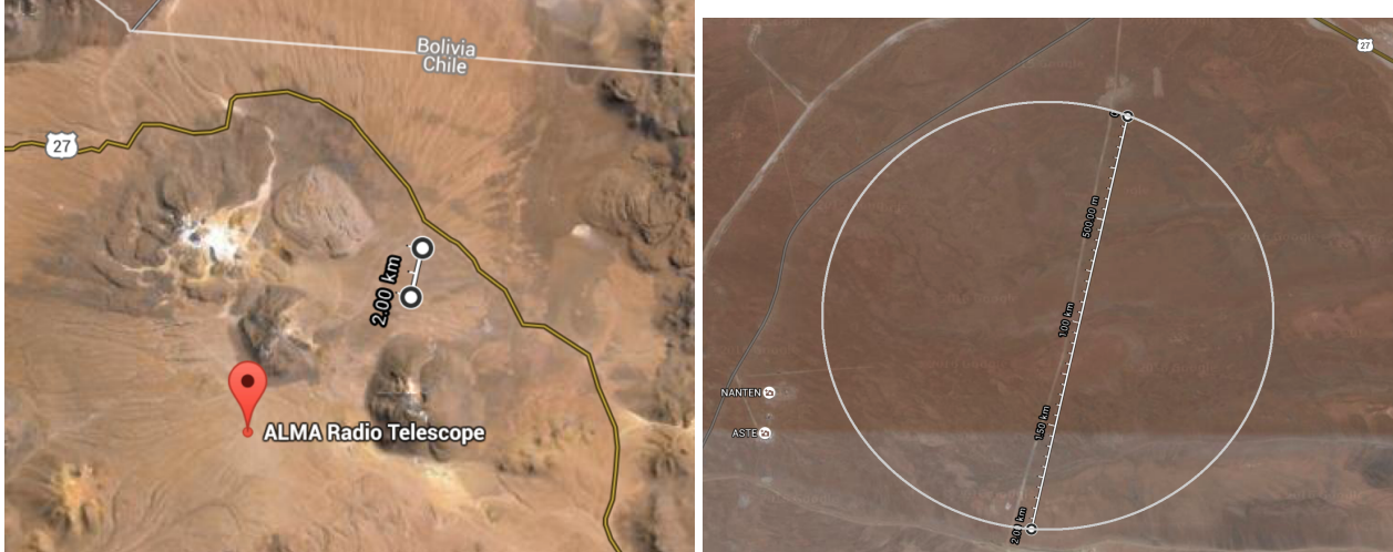
Figure 1. An example suitable site for PFI, next to the ALMA observatory. This site has low water vapour (essential for \sim 5 \mu\text{m} observations) and sub-arcsecond seeing expected. With a circular array geometry, pylon heights would be less than 10 m.
