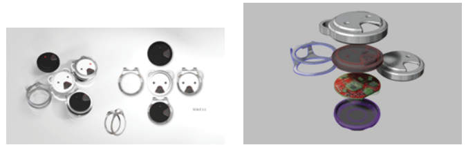
(a) Koala beacon used as Dumb Toy. (b) Koala beacon inner component.
